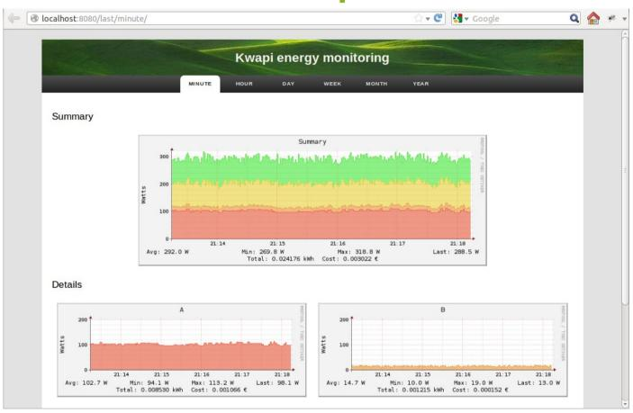
The Kwapi visualization plugin allows to monitor the power consumption of compute nodes.
