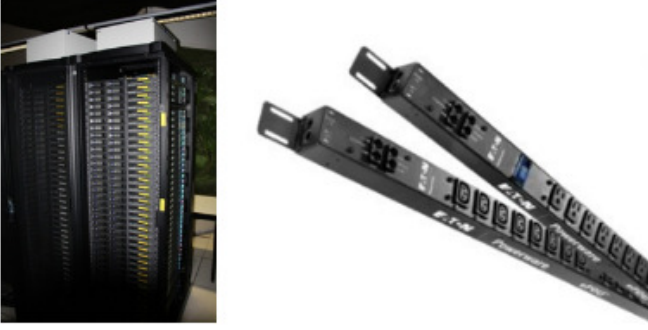
Fig. 1. (Left) Prototype of wattmeter made by OmegaWatt for monitoring 150 nodes in our data center. (Right) Outlet power strip (ePDU) which allow to query each outlet individually.
