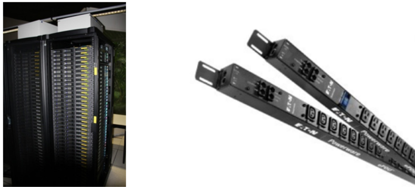
Figure 1: (Left) Prototype of wattmeter made by OmegaWatt for monitoring 150 nodes in our data center. (Right) Outlet power strip (ePDU) which allow to query each outlet individually.
